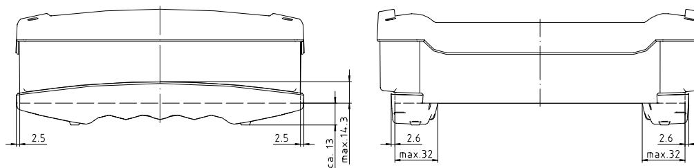
Different bow ends ensure that the subsequent „parking position“ of the bow can be set during assembly.
