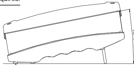
Optional rubber foot assembly for additional support (included in scope of delivery).
